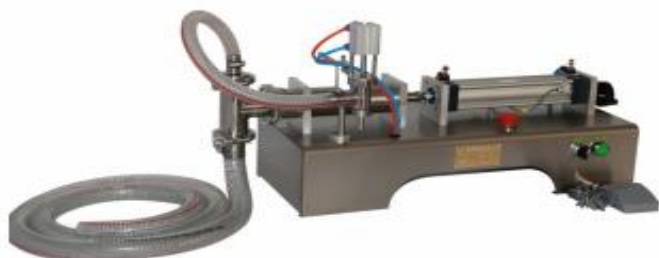
Single nozzle liquid filling machine (GT-SY)
